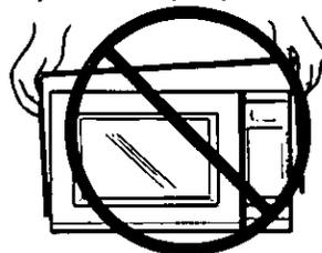
2. Do **NOT** operate the oven empty. The microwave energy will reflect continuously throughout the oven if food or water is not present to absorb energy. This could damage the oven and result in the danger of a fire.
