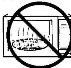
3. Do **NOT** use this oven to heat chemicals or other non-food products. Do **NOT** clean this oven with any product that is labeled as containing corrosive chemicals. **The heating of corrosive chemicals in this oven can cause radiation leaks.**
