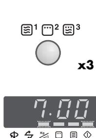
3. Choose the desired power by rotating the **TIMER/WEIGHT/POWER** knob clockwise.
