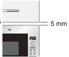
5. Fix the oven in position with the screws provided. The fixing points are located on the top and bottom corners of the oven (see diagram, item 10, on page 5).
