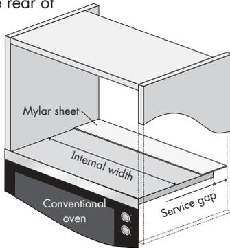
3. Fit the appliance into the kitchen cupboard slowly, and without force, until the front frame of the oven seals against the front opening of the cupboard.
