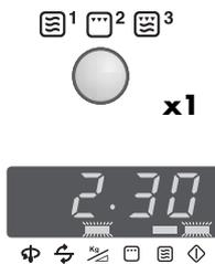
3. Choose the desired power by rotating the **TIMER/WEIGHT/POWER** knob clockwise.
