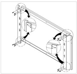
For the bracket assembly, locate parts properly by distinguishing them using inlayed L(left), R(right), TOP (top), and BOT(bottom) markings.
