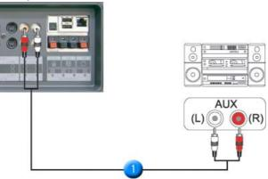
Connect a set of audio cables between the AUX L, R jacks on the AUDIO SYSTEM and the MONITOR [R-AUDIO-L] on the Monitor.
