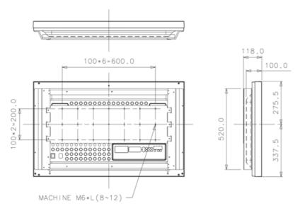
For securing the bracket on a wall, use only machine screws of 6 mm diameter and 8 to 12 mm length.
