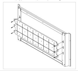
Secure the bracket onto the backside of the LCD Monitor using screws.
