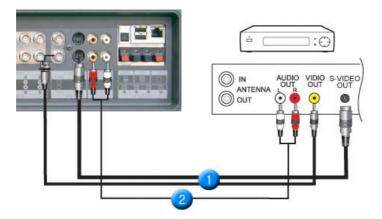
AV input devices like VCRs or Camcorders are connected to the AV IN [VIDEO] or AV IN [S-VIDEO] of the monitor using the S-VHS or BNC cable.
