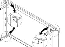
Fix the VESA Bracket onto the assembled Main Bracket. Be sure that the VESA Bracket is placed correctly not to confuse front and back side of the VESA bracket. Machine Screw(2)
