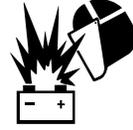
• **CONNECTING A BATTERY CHARGER** - Remove battery from welder by disconnecting negative cable first, then positive cable and battery clamp. When re-installing, connect negative cable last. Keep well ventilated.
