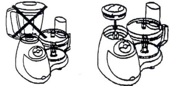
**WARNING:** The food processor bowl must always be in place with the food processor lid in place when using the blender. Please note that **NO** accessory (i.e. blade or attachment) must be inserted inside the food processor bowl when the blender is being used.
