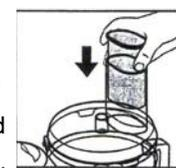
**For safety, always use the food pusher when putting food into the feeder tube. Never feed by hand. (Fig. 9)**
