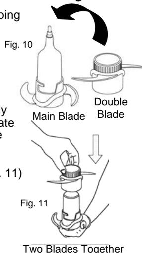
2. Then insert onto the shaft of the processor bowl. Always hold the chopping blade by the upper plastic part. (Fig. 12)
