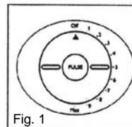
Use of the Pulse/Turbo button allows greater control over the texture of the food being processed. Use "Pulse" when the unit is in the "Off" position. Use "Turbo" when the unit is in the "On" position and you need a burst of power. Please note that the "Pulse" and "Turbo" is only intended to be used for short "bursts" of processing.
