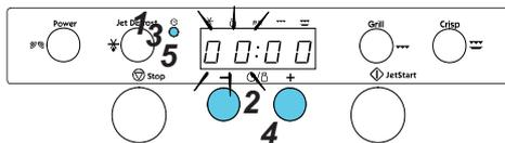
**Keep the door open** while setting the Clock.
