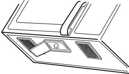
3. Replace light. Close bulb cover. Replace mounting screws.
