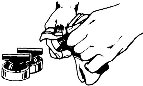
3. Wash knobs and surface unit collars in warm soapy water. Rinse well and dry.
