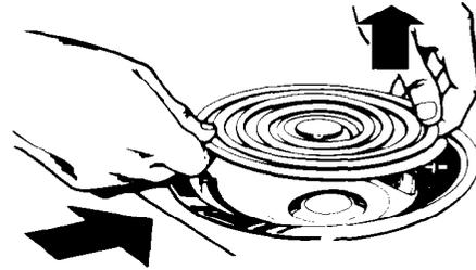
4. While pushing the surface unit terminal into the receptacle, lift a little on the edge of the unit nearest the receptacle.
