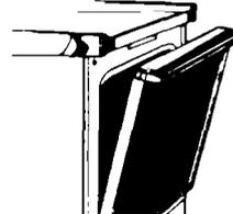
5. During broiling, the oven door must be partly open. A built-in stop will hold it there.
