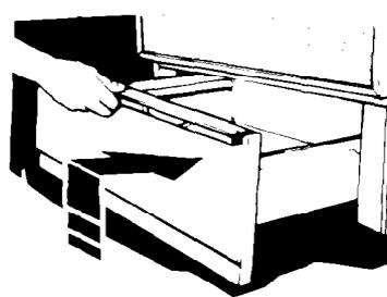
2. Lift drawer front and push in until metal stops (on drawer slide rails) clear white stops on drawer guides.
