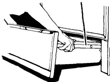
1. Fit ends of Drawer Slide Rails into drawer guides on both sides of opening.
