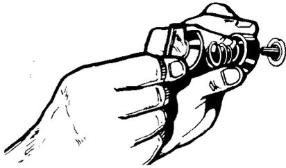
1. First make sure lower oven and surface unit control knobs are set on OFF. All knobs pull straight off. Surface unit knobs have a collar and spring.
