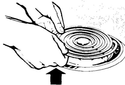
2. Lift the edge of the unit opposite the receptacle just enough to clear the reflector bowl.
