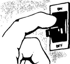
1. Turn off the electric power at main power supply.
