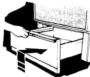
3. Lift drawer front to clear second stop and slide drawer closed.
