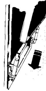
Fit the bottom corners of the door over the ends of the hinges.
