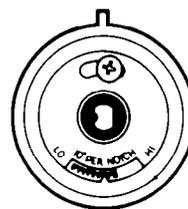
3. To lower the temperature, move black part of knob closer to **LO**. Each notch equals about 10°F (5°C).
