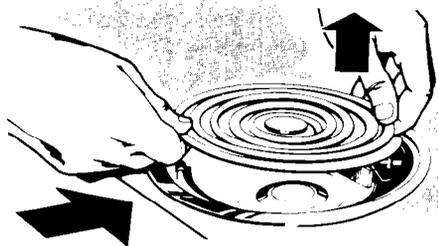
4. While pushing the surface unit terminal into the receptacle, lift a little on the edge of the unit nearest the receptacle.
