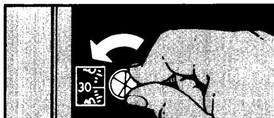
2. Without pushing in, turn the knob back so the setting you want shows in the window.
