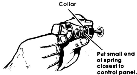
4. Push knobs straight back on. Make sure they point to OFF. Make sure the collar and spring on surface unit knobs are put together as shown.
