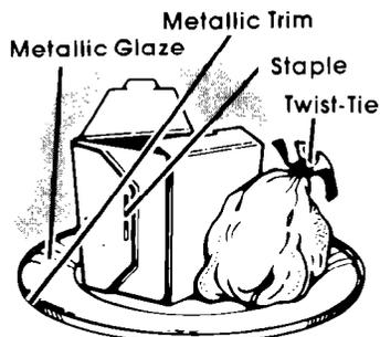
Cooking in metal containers **can damage the oven**. So can containers with **hidden metal** (twist-ties, foil-lining, staples, metallic glaze or trim). *Test dinnerware or cookware before using.*
