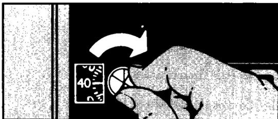
1. Without pushing in the Minute Timer Knob, turn it until the time showing in the window is longer than you want.
