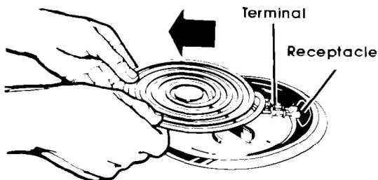
3. Pull the surface unit straight away from the receptacle.
