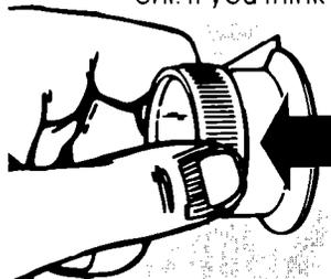
1. Pull the Oven Temperature Control straight off.
