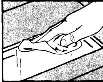
**WINDOW** – Keep clean with hot sudsy water. Do not use steel wool or abrasive cleansers. Use a plastic scouring pad for stubborn spots. Rinse well.
