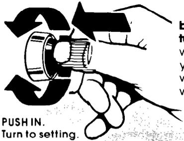
**Control knobs must be pushed in before turning.** Turn either way until the setting you want shows in the window. Set them anywhere from HI to OFF.
