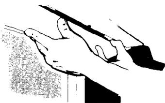
7. Slide the cover back far enough for the front to fit behind the spring tabs at the ends.
