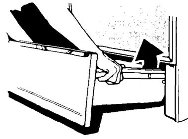
3. Lift back slightly and slide drawer all the way out.
