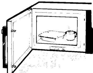
*To test a dish for safe use, put it into the oven with a cup of water **beside** it. Cook on high Cook Power for one minute. **If the dish gets hot and the water stays cool, do not use it.***
