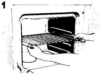
Lift rack at front and pull out.
