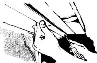
2. Remove the 3 screws and front metal trim that supports the light cover. **The glass is heavy. Hold it securely.**
