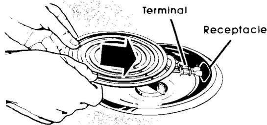
3. Hold the surface unit as level as possible with the terminal just started into the receptacle.
