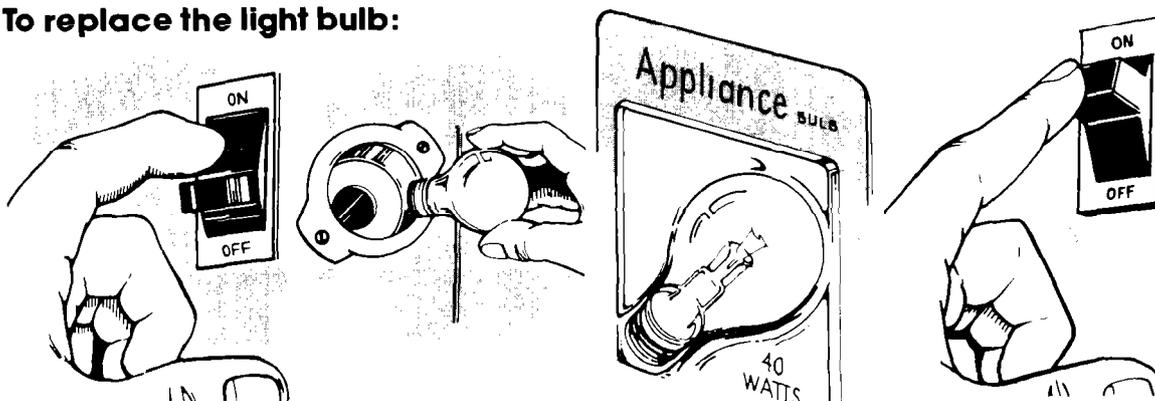
1. Turn off the electric power at the main power supply.
