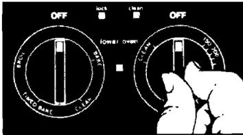
7. After baking is done, turn both knobs to OFF
