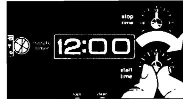
3. Push in and turn the Start Time Knob **clockwise** to the time you want baking to start.
