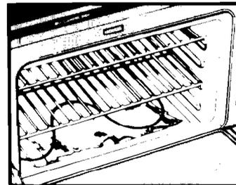
**DO NOT** use foil or other liners in the oven. During the cleaning cycle, foil can burn or melt.
