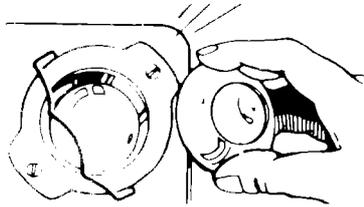
2. Remove the bulb cover by pulling out on the wire holder and moving it to the side.
