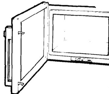
It is normal for the inside of the oven door to look wavy after the oven has been running for a while.
