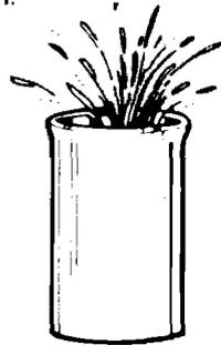
Liquids heated in certain containers may overheat. The liquid may then splash out with a loud noise. This does not harm the oven, but you should not use such containers to heat liquids again.
