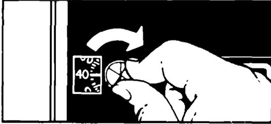
1. Without pushing in the Minute Timer Knob, turn it until the time showing in the window is longer than you want.
