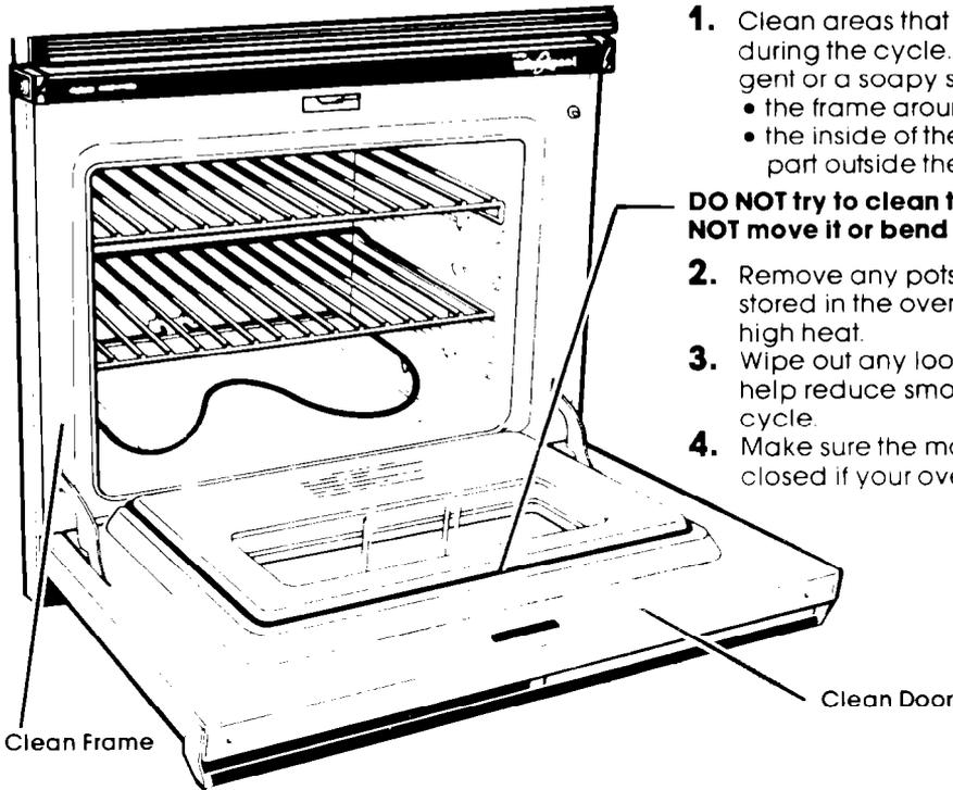
1. Clean areas that may not be cleaned during the cycle. Use hot water and detergent or a soapy steel-wool pad on...
