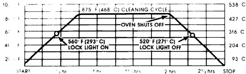
Note: The heating stops when the two-hour setting is up, but that it takes a while longer for the oven to cool down enough to unlock.
