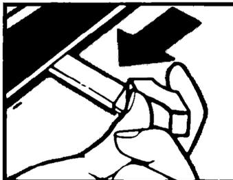
**DO NOT** force the Lock Lever. The lever is designed to stay locked until the oven is cool enough to safely open.
