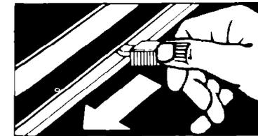
9. Move the Lock Lever back to the left. **Do not force it.** Wait until it will move easily. This turns off the Clean Light.
