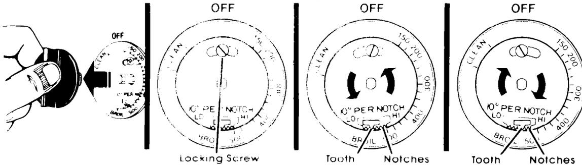
1. Pull out the center of the Oven Temperature Control.
