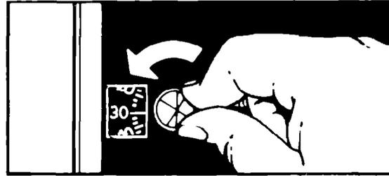
2. Without pushing in, turn the knob back so the setting you want shows in the window.
