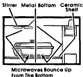
The food container rests on a sealed-in ceramic shelf above the metal bottom of the oven cavity. Because the food is above the metal bottom, microwaves can get under it, through the ceramic shelf, to bounce up from the bottom into the food.
