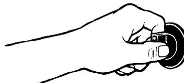
2. Lift the edge of the unit, opposite the receptacle, just enough to clear the reflector bowl.
