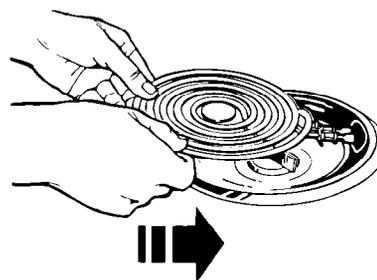
4. When terminal is pushed into the receptacle as far as it will go, push down the edge of the surface unit opposite the receptacle.
