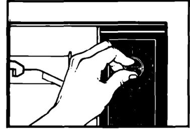
3. Set the cooking time by turning the Timer Knob clockwise. To reduce the cooking time, turn the Timer Knob counterclockwise. **To set timer for less than 1 minute, turn timer past 1 minute then to desired time.**
