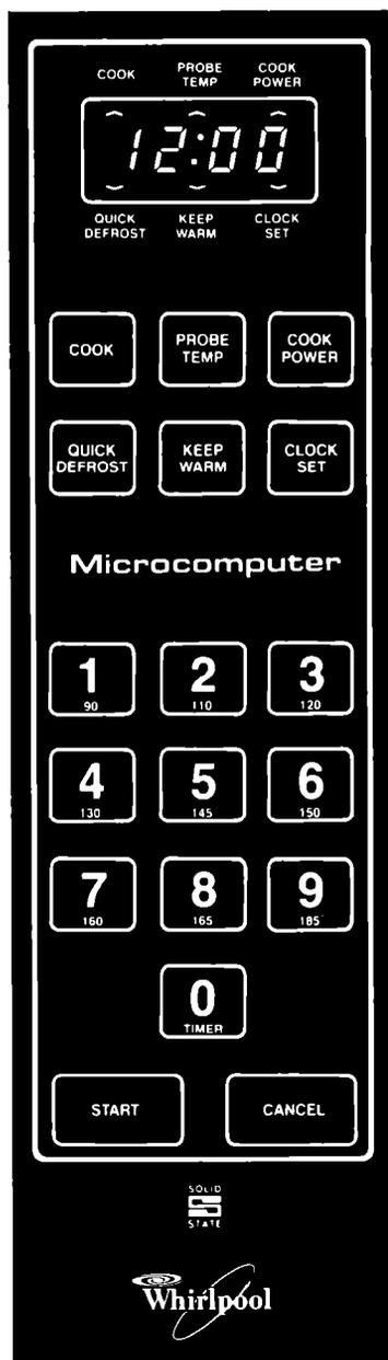
When you first plug in the oven, the Display will show 88:88. If, after you set the Clock (page 6), the Display again shows all 8's, it means your electricity was off for a while. Reset the Clock.
