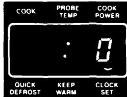
The **CLOCK SET** Indicator Light will come on. The Display will show a "0." **Start touching number pads for the desired time within 5 seconds.**
