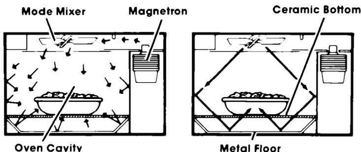
A magnetron in the microwave oven produces microwaves. The microwaves move into the oven where they are scattered or stirred by a mode mixer (like a fan). Microwaves bounce off metal oven walls and are absorbed by food.
