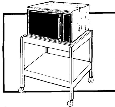
**2.** Put the oven on a cart, counter, table or shelf that is strong enough to hold the oven, the food and the utensils you put in it. **(The control side of the unit is the heavy side. Use care when handling.)** The weight of the oven is approximately 60 lbs. (27 kg).
