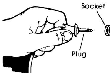
**2.** Place food in the oven and plug the probe into the socket on the oven wall.
