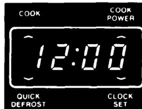
When you are not using the microwave oven, this is an accurate digital clock. When you are using the microwave oven, this displays time and Cook Power settings, indicator lights and shows you what Number Pads you touched.
