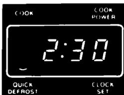
When you touch **START**, the **QUICK DEFROST** Indicator Light will stay on. All other Indicator Lights will go off. The Display counts down the time to show how much time is left in the defrost cycle.
