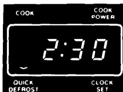
The QUICK DEFROST Indicator Light will stay on to show that the oven is in the QUICK DEFROST cycle.
