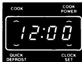
When you are not using the microwave oven, this is an accurate digital clock. When you are using the microwave oven, this displays time and Cook Power settings, signal lights and shows you what Number Pads you touched.
