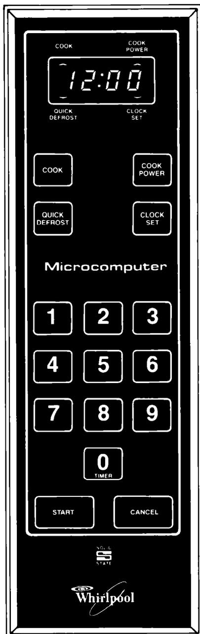
When you first plug in the oven, the Display will show 88:88. If, after you set the Clock (page 6), the Display again shows all 8's, it means your electricity was off for a while. Reset the Clock.
