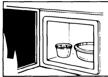
To test a dish for safe use, put it into the oven with a cup of water **beside** it. Cook on high Cook Power for one minute. **If the dish gets hot and water stays cool do not use it.**
