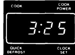
The Clock is set when the **CLOCK SET** Signal Light goes off.
