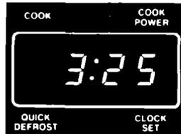
The Clock is set when the **CLOCK SET** Signal Light goes off. The Display will flash on and off if you have touched in an incorrect time such as 12:65.
