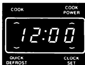
When you are not using the microwave oven, this is an accurate digital clock. When you are using the microwave oven, this displays time and Cook Power settings, signal lights and shows you what Number Pads you touched.
