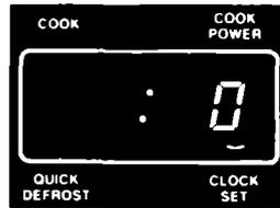
The **CLOCK SET** Signal Light will come on. The Display will show a "0." **Start touching number pads for the desired time within 5 seconds.**
