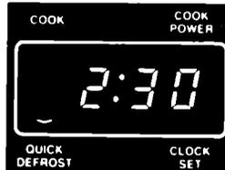
The QUICK DEFROST Signal Light will stay on to show that the oven is in the QUICK DEFROST Cycle.
