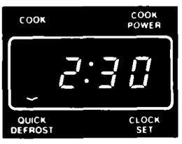
When you touch START, the QUICK DEFROST Signal Light will stay on. All other Signal Lights will go off. The Display counts down the time to show how much time is left in the defrost cycle.
