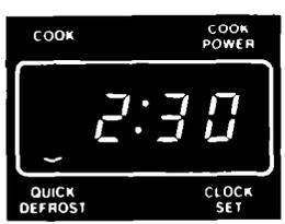
When the defrost time ends, the microwave oven automatically lets the food stand for the **same amount of time used for defrosting**. The QUICK DEFROST Signal Light stays on and the Display counts down the standing time. **During the count-down the oven will be dark, and the fan will be off.**
