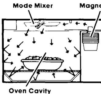
A magnetron in the microwave oven produces microwaves. The microwaves move into the oven where they are scattered or stirred by a mode mixer (like a fan). Microwaves bounce off metal oven walls and are absorbed by food.
