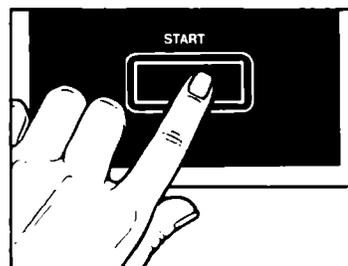
**5.** Push the START Button. The oven light will come on and cooking will begin. You will hear the fan running during oven operation.
