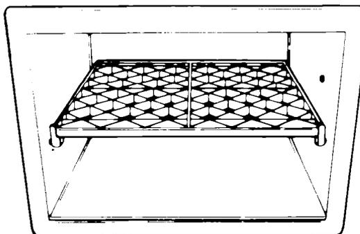
**Second Position:** Turn rack upside-down when using a taller container on the bottom of the oven.
