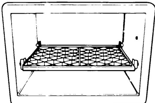
**First Position:** Use the rack only when heating more than one container of food. **Do not let a container touch the top or sides of the oven.**
