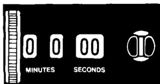
The timer can be set for up to 59 minutes, 55 seconds. This controls how long the microwave oven cooks.
