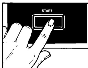
**6.** Push the START Button. When the probe senses the temperature you selected, a beep sounds, and the oven shuts off.
