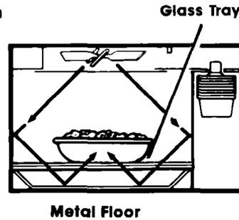
The glass tray of your microwave oven lets microwaves through. Then they bounce off a metal floor, back through the ceramic bottom and are absorbed by the food.
