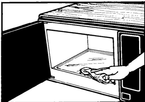
**1.** Empty the microwave oven and clean inside it with a soft, damp cloth. Check for damage such as misaligned door, damage around the door or dents inside the oven or on the exterior. If there is any damage, please do not operate the unit until it has been checked by an authorized Whirlpool service technician and any repairs have been made.
