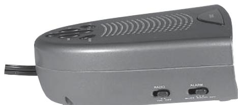
1. Make sure the radio is off by setting **RADIO ON/OFF** to **OFF**.
