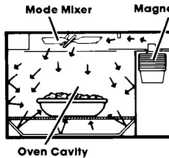
A magnetron in the microwave oven produces microwaves. The microwaves move into the oven where they are scattered or stirred by a mode mixer (like a fan). Microwaves bounce off metal oven walls and are absorbed by food.
