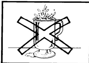
Liquids heated in certain containers (especially cylindrical-shaped containers) may become overheated. The liquid may splash out with a loud noise during or after heating or when adding ingredients (coffee, etc.) resulting in harm to the oven and possible personal injury. For best results stir any liquid several times before heating or reheating.
