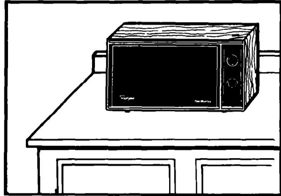
**2.** Put the oven on a cart, counter, table or shelf that is strong enough to hold the oven and the food and utensils you put in it. **(The control side of the unit is the heavy side. Use care when handling.)** The weight of the oven is approximately 43.5 lbs. (19.57 kg.).
