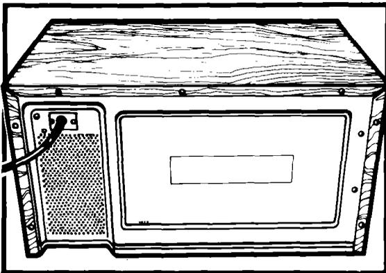
**3.** Do not block the front vent or rear air intake openings. Blocking vent or air intake openings can cause damage to the oven and poor cooking results. Make sure the microwave oven legs are in place to ensure proper air flow.
