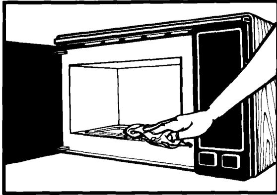
**1.** Empty the microwave oven and clean inside it with a soft, damp cloth. Check for damage such as misaligned door. Damage around the door or dents inside the oven or on the exterior. If there is any damage, **do not** operate the unit until it has been checked by an authorized Whirlpool service technician and any repairs have been made.
