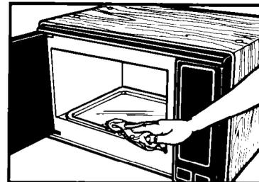
**Be sure to keep the areas clean where the door and oven frame touch when closed.** Use only mild, non-abrasive soaps or detergents applied with a sponge or soft cloth when cleaning surfaces of door and oven that come together. Rinse well.
