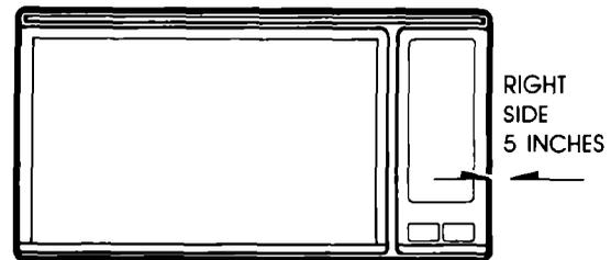
**4.** Do not install the microwave oven so that any part of it is flush with a wall, shelf or cabinet. Leave a total clearance of at least 5 in. (12.7 cm) around the oven for proper operation.
