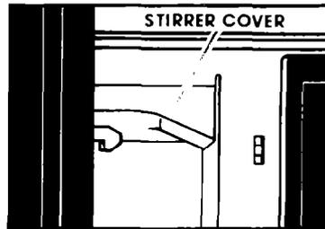
**NEVER** remove the stirrer cover. The plastic cover protects the microwave stirrer blade from soil or bending.
