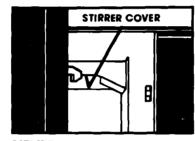
**NEVER** remove the stirrer cover. The plastic cover protects the microwave stirrer blade from soil or bending.
