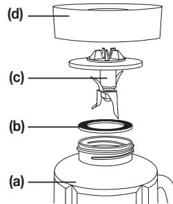
2. Position the rubber gasket (b) on the round opening on the bottom of the blender jar.
