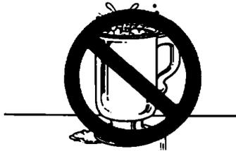
Liquids heated in certain containers (especially cylindrical-shaped containers) may become overheated. The liquid may splash out with a loud noise during or after heating or when adding ingredients (coffee, etc.) resulting in harm to the oven and possible personal injury. For best results stir any liquid several times before heating or reheating.
