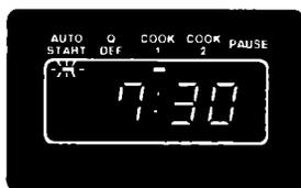
5. Touch START. The present time of day will show in the display window, the AUTO START Indicator Light will blink and the COOK 1 Indicator will stay on. As soon as the clock shows the preset cook start time, the oven will start cooking and the Display will count down the set time.
