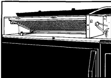
8. Slide a new charcoal filter into place. The filter should rest at the angle shown.
