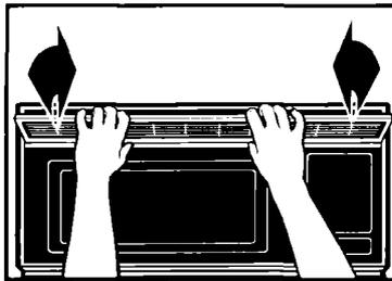
9. Slide the bottom of the vent cover into place. Push the top until it snaps into place. Replace the mounting screws.
