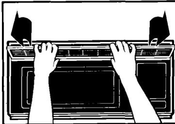
5. To replace charcoal filter: remove the vent cover mounting screws.
