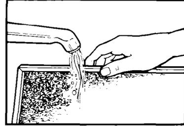
3. Soak grease filters in hot water and a mild detergent. Scrub and swish to remove embedded dirt and grease. Rinse well and shake to dry. **Do not use ammonia or place in a dishwasher. The aluminum will darken.**
