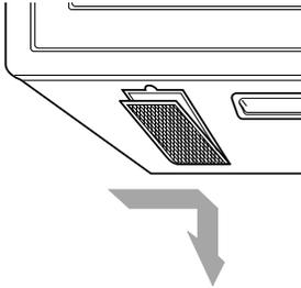
3. Remove charcoal filter by removing the vent grille mounting screws, tipping the grille forward and lifting out to remove. Open the microwave oven door. Then press the tab and lift the front of the filter up, and slide filter straight out.
