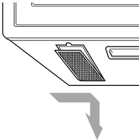
3. Remove charcoal filter by removing the vent grille mounting screws, tipping the grille forward and lifting out to remove. Then lift the front of the filter up, and slide filter straight out.
