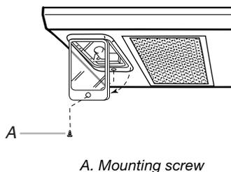
3. Replace light. Close bulb cover. Replace mounting screw.
