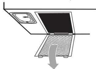
3. With the tab side of the new or cleaned filter facing down, insert the end without the tab into the frame, then swing the end with the tab up and slide the filter into place.
