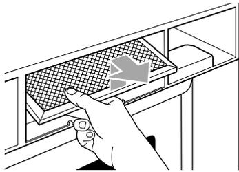
4. Slide the new filter back and into place so that it rests at an inclined angle (about 45°).
