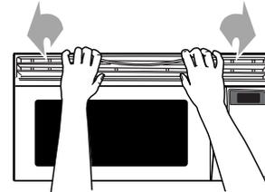
3. Remove the charcoal filter (see “Replacing Filters” section).
