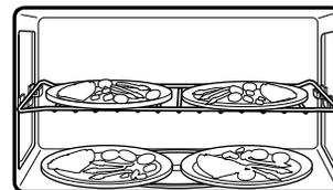
The turntable must be turned off while heating 2 bottom plates or 1 larger dish. See "Turntable" section.
