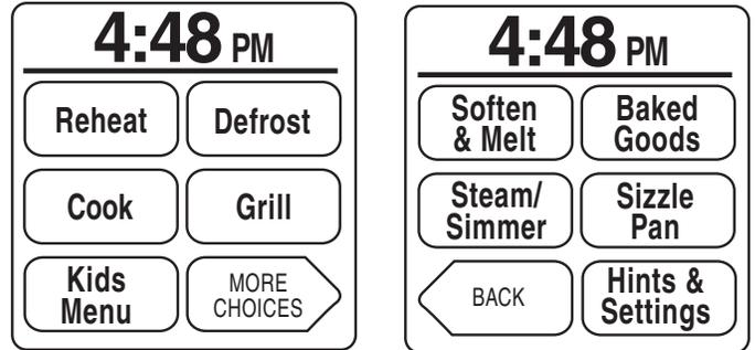
The LCD touch screen is used to input commands. A light- to medium-pressure touch of the fingertip will activate the menu choice. However, sensitivity of the touch screen may vary, and using the tips or backs of fingernails may provide more accuracy when inputting commands.
