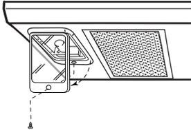
3. Remove the burned-out bulb.
