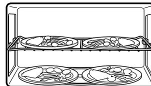
The turntable must be turned off while heating 2 bottom plates or one larger dish. See "Turntable" section.
