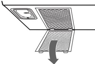
3. Remove each charcoal filter by pushing the filter toward the center of the oven until it is clear of the narrow outer lip. Swing the filter down and slide it out.
