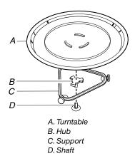
The turntable can rotate in either direction to help cook food more evenly. Do not operate the oven without the turntable in place. See "Assistance or Service" to reorder any of the parts.
