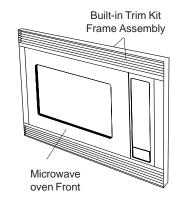
For installation with a gas (VGS0166) or electric (VES0165) 36" wide single oven use built-in trim kit VMTK360SS.
