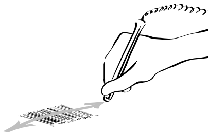
Figure 4. Scan the entire barcode from left to right beginning outside the left edge then back across it right to left.
