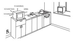
A minimum clearance of 3.0 inch (7.5cm) is required between the oven and any adjacent wall. One side must be open.
