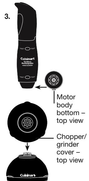
4. With the hand blender in place, locate the chopper/grinder cover and place it on top of the prep bowl.
