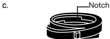
Pick up the blade ring by its hub holding ribs (grips) and line up the notches in the interior of the blade ring hub with the ridges on the sides of the plastic blade sheath. Let the blade ring slide down to the bottom of the plastic blade
