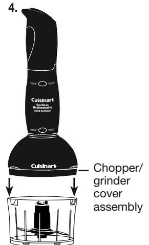
the prep bowl. Rotate cover counterclockwise to secure it to the prep bowl. Rotate the cover until the pins are in the far left position in the slots.
