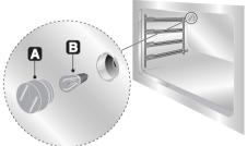
Remove the bulb protector A by turning it anticlockwise and replace bulb B with a similar one (25 W). Re-fit the bulb protector A.
