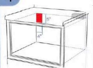
Place electrical outlet in upper back left side in the cavity opening. Can also be installed using an electrical outlet in an adjacent cabinet. Always check electrical codes for requirements.
