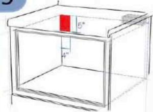
Place electrical outlet in upperback left side of opening. Electrical outlet can also be placed in an adjacent cabinet. Always check electrical codes for requirements. Proceed to Installation Instructions to install Drawer into cabinet.
