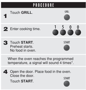
If the oven door is not opened, the oven will automatically hold at the preheat temperature for 30 minutes. After this time has elapsed, an audible signal will sound and the oven will turn off.
