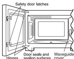
Check the oven for any damage, such as misaligned or bent door,
