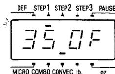
**NOTE:** Since the oven temperature is 350°F in this case, the temperature need not be entered since this temperature is preset in the oven.
