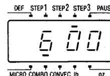
**NOTE:** During convection cooking, the oven keeps the same temperature in second stage as for preheating. If, however, the third stage is used, and a temperature other than 350°F is desired, the oven temperature must be set in third stage.
