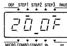
After the oven reaches the preheat temperature a “beep” tone will sound. The oven is now preheated.
