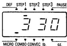
Remember, the timer is a digital clock that is divided into 60 seconds. Therefore, 1/2 minute is equal to 30 seconds. Touch 30 and not 50 (as with a calculator) to indicate 1/2.
