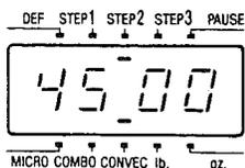
The temperature selected in the preheat stage (first stage) will be maintained in the convection cooking stage (second stage). However, if a third stage is used and a temperature other than 350°F is desired, the oven temperature must be set for this third stage.
