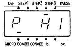
8. To set power level 20, touch and HOLD "LOW" PAD until "P 20" appears in the display window.
