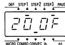
When the temperature reaches 350°F, “350F” shows in the display window and a “beep” tone will sound to indicate that the preheating time is over.
