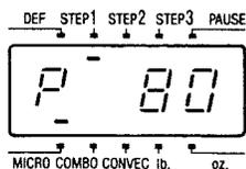
**NOTE:** When using the LOW/HIGH PADS to change power levels you can touch them once, or twice, etc., or you can touch and hold the pad. The display window will show the power levels changing automatically.
