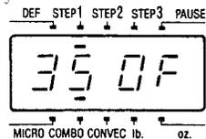
3. Set the desired oven temperature, if different than the preset 350°F.
