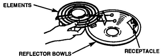
**CAUTION:** Do not pull element up more than 1/2" or damage to the receptacle will occur.
