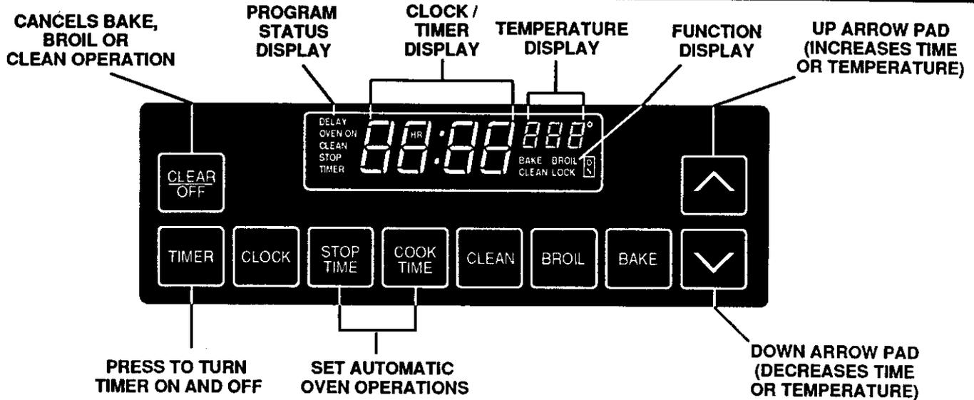
Your range control is touch controlled. To set BAKE, BROIL, TIMER or CLEAN, touch the desired function pad and select the temperature or time by touching the arrow pad.
