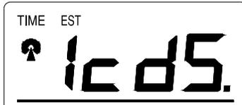
**Note:** There are 8 LCD contrast levels to choose from—“Lcd 0” is the lightest, and “Lcd 7” is the darkest.
