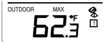
3. While “MAX” is still displayed press the *OUT* button again to return to the current data display. Or you can wait 30 seconds, during either the minimum or the maximum readings, and the unit will automatically return to current data readings.
