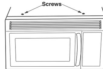
Remove 2 grille screws to remove the grille
