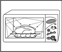
1. The microwaves generated by the magnetron are distributed uniformly as the food rotates on the turntable. The food is thus cooked evenly.
