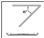
When cleaning the upper part inside the cavity, it will be convenient to turn heater downward by 45° and clean it.
