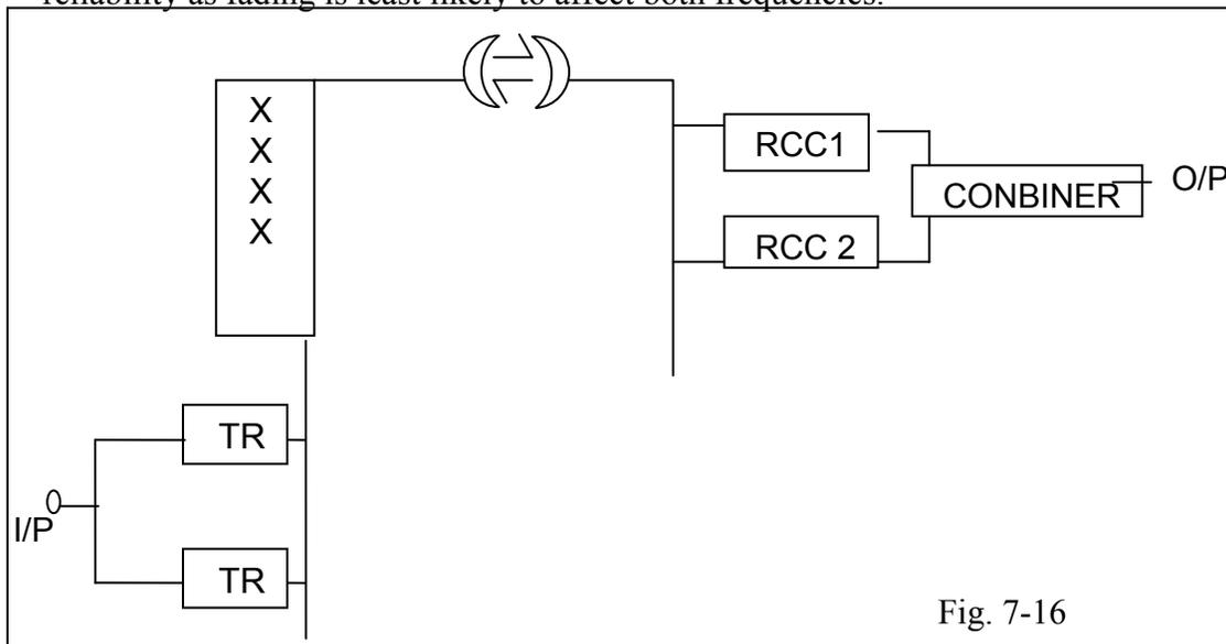
3. Space diversity: - It is applicable in W/B system for larger hops. Each site is provided with two Antennas. Main antenna at station A transmits signals of all frequencies, at station B signal received by both antennas main and space diversity which will detect the signal with lowest path loss between two sites.
