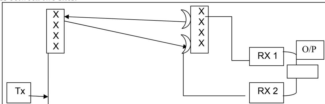
Antenna diversity: - In this diversity scheme microwave signals are transmitted along with different propagation path with the help of second antenna at receiving end to improve received performance.
