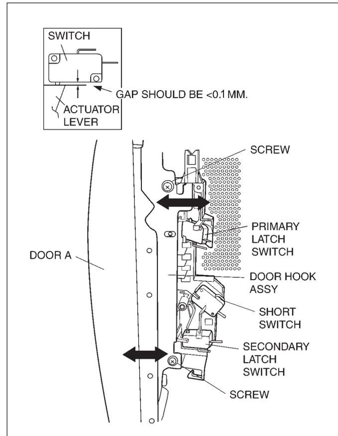
Please confirm that the gap between the switch housing and switch actuator lever is no more than 1.0mm when the door is closed.
