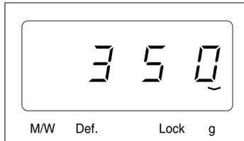
When you press REHEAT MEAL button, "350" is displayed. The g indicator lights. After the 1.5 seconds, the display changed into cooking time of quantity and the oven starts cooking. The g indicator goes off.
