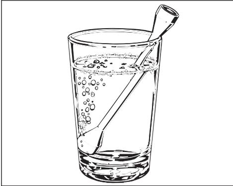
When heating liquids, milk, sauces etc. in the oven without the boiling rod, the boiling point of the liquid may be reached without the production of typical bubbles. The liquid does not boil evenly throughout. This so-called 'boiling delay' can cause a sudden build-up of bubbles when the container is removed from the oven or shaken, which can lead to the liquid boiling over suddenly and explosively. Danger of burning.
