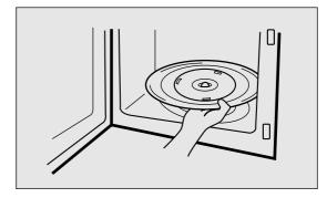
7 The roller guide and oven cavity floor should be cleaned regularly to avoid excessive noise. Simply wipe the bottom surface of the oven with mild detergent water or window cleaner and dry. The roller guide may be washed in mild sudsy water.
