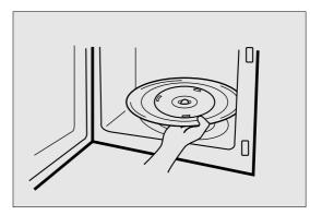
7 The roller guide and oven cavity floor should be cleaned regularly to avoid excessive noise. Simply wipe the bottom surface of the oven with mild detergent water or window cleaner and dry. The roller guide may be washed in mild sudsy water.
